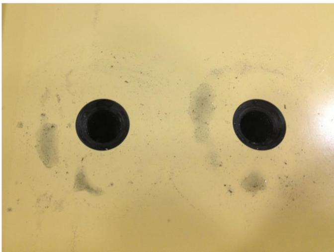
Figure 11. Holes with cutting fluid and debris used for the repeatability assessment.
