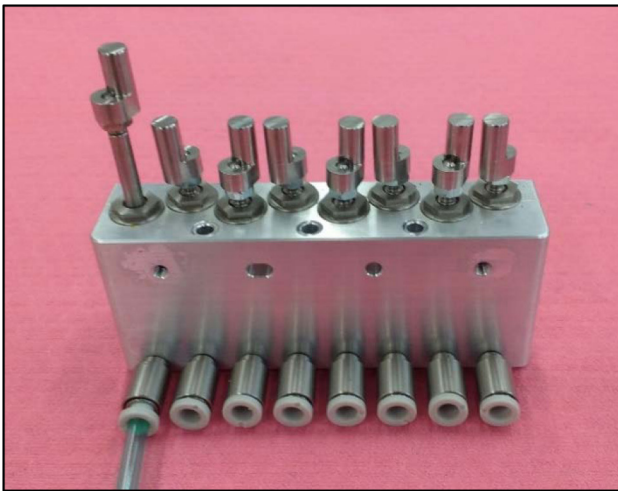
Figure 12. Fastener Escapement Cylinder Assembly; 8 Air Cylinders.
